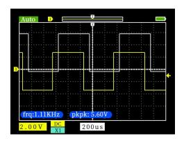
11.Waveform screenshot: Click in the button panel key, Capture the current screen and save. You can save up to 81 screenshots (9 pages in total, 9 per page), If there are more than 81 sheets, the oldest sheet will be replaced. You can delete unnecessary pictures.
