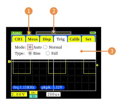
**1.**Switch by SEL button, Move the joystick up and down to move the vertical offset, Trigger position.
