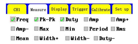
They are frequency, peak-to-peak value, positive duty cycle, amplitude, positive amplitude, negative amplitude, maximum, minimum, period, root mean square, average, positive pulse width, negative pulse width, and negative duty cycle
