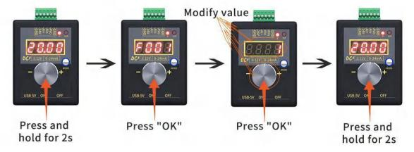
Figure  $1\rightarrow 2$ : Press and hold the knob for 2 seconds, Enter setting state, Display "F001";
