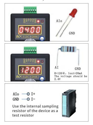
7.2 Connect an LED indicator, if the brightness changes with the adjustment, then the signal generator current output is no problem; 7.3 Connect a 50-300
